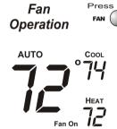
Fan On indicates constant fan operation. This feature is active even if the thermostat is set to Off.
