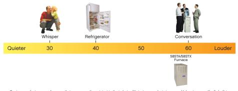
Carrier manufactures gas furnaces that are among the quietest in the industry. We test our products in a sound laboratory specifically built to resemble a typical residence. Sound level recordings produced at steady state, single-stage operation (the most common operating condition) measured 3 feet from furnace. Other sound levels, mentioned for comparison, as published at http://www.nidcd.nih.gov/heaith/hearingr.uter.asp.
