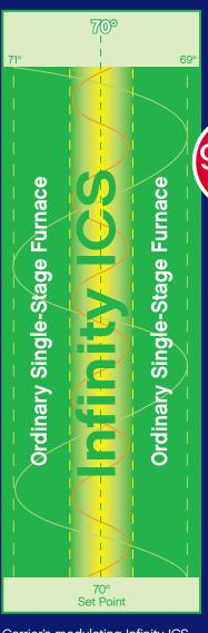
Carrier's modulating Infinity ICS gas furnace minimizes temperature "swings" to deliver comfort within a tighter range of degrees from your set temperature.
